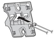
2 Tuck the telephone line cord inside the wall mounting adaptor (1). Connect the AC adaptor cord and telephone line cord (2).
